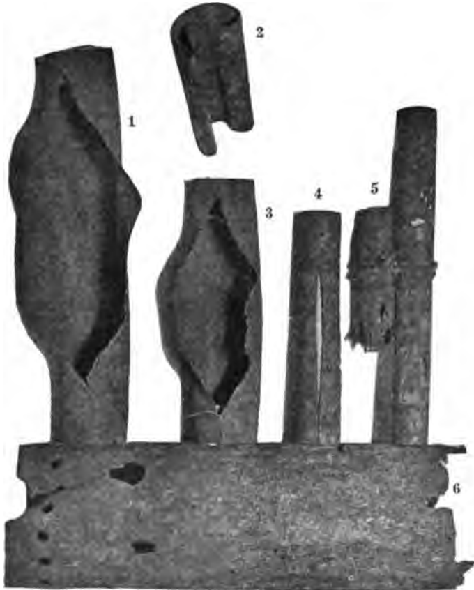
FIG. 18.—Nos. 1 and 3, Ruptured Tubes; No. 2, Collapsed Tube; 4, Split Feed-pipe; 5, Corroded Tubes. No. 6 was taken from a water-tube boiler and carried 100 pounds of steam up to the time inspection was made. Accumulation of scale inside prevented its leaking.
